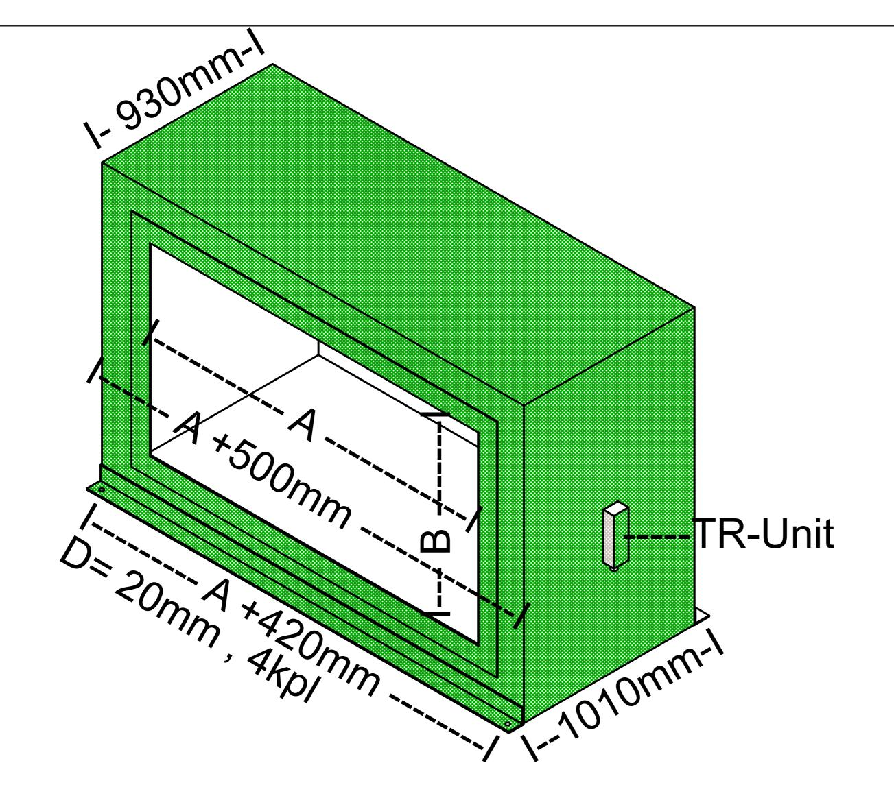
TC-coils have been protected against the influence of metallic constructions on all sides of the coil by a rigid aluminium body. The sensitive coils have been located very close to the inner surface under
